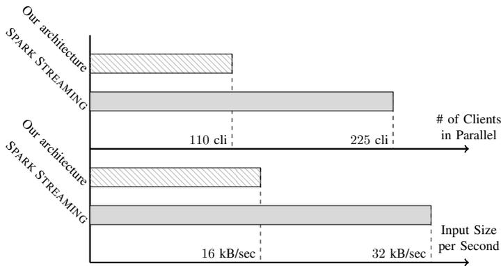
Fig. 3. Comparison of the maximum number of clients served in parallel and the maximum input load between the proposed architecture and SPARK STREAMING. (Left) Proportional bar representation of the values at which each system becomes unstable: it can not process the input received during the past 10 seconds in under 10 seconds. (Right) Summary table of the same values.
